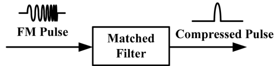
Fig. 1. Basic principle of pulse compression with frequency modulation (FM).
